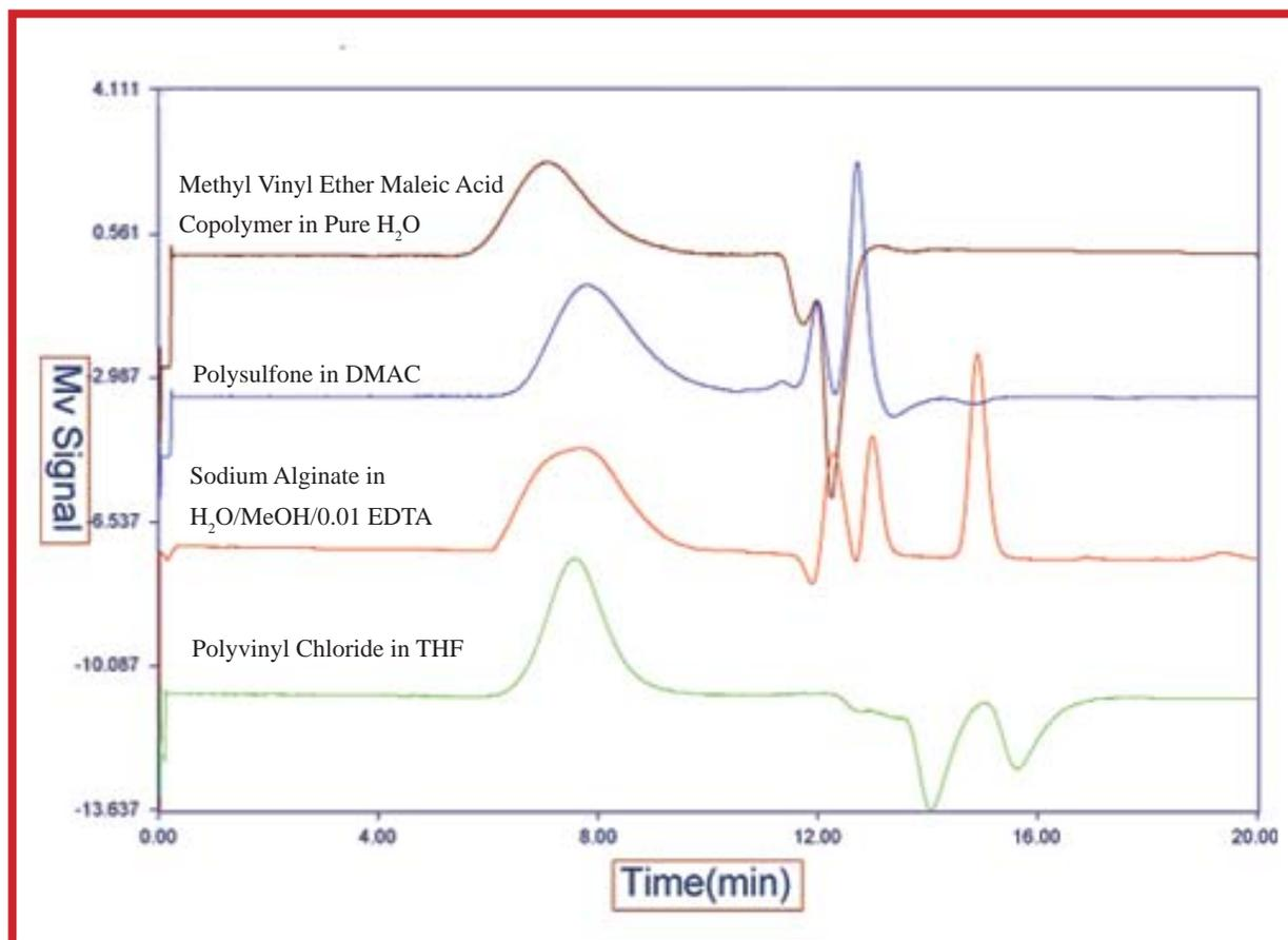
*\*Chromatogram above shows four analytes run on a single Jordi xStream H<sub>2</sub>O™ Mixed Bed Column in an appropriate mobile phase.*
