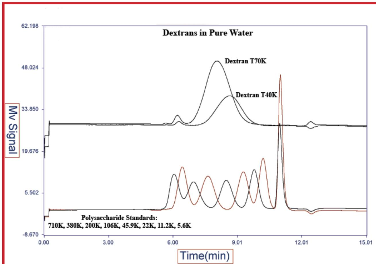
The Jordi xStream H<sub>2</sub>O™ affords versatility and efficiency to any GPC lab. This polyamide-based technology allows for various separations on the same column set. Using a suitable solvent changeover procedure, one can easily switch solvents without damaging the stationary phase. The highly cross-linked nature of our novel, polyamide-based packing material reduces swelling and shrinking, which provides high resolution in nearly all solvents and promotes longer column lifetime.
